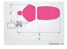
Particularly suitable for orthodontists: a single satellite is fixed to the rear of the chair in a position suitable for right- and left-handed practitioners that uses pneumatic technology to drive dynamic instruments. A maximum of six instruments can be fitted to this stand: suction tube, syringe, turbine, pneumatic or electric micromotor, plaque remover, polymerising lamp, camera, etc. as required.
